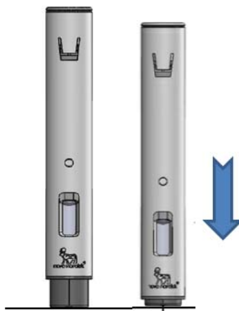
Figure 10 Activation of the single dose pen-injector for semaglutide by pressing the exposed Needle cover against the skin
