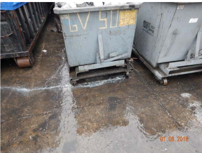
Photo 5. Cutting fluid from the shavings in the bin leaking onto the ground.
