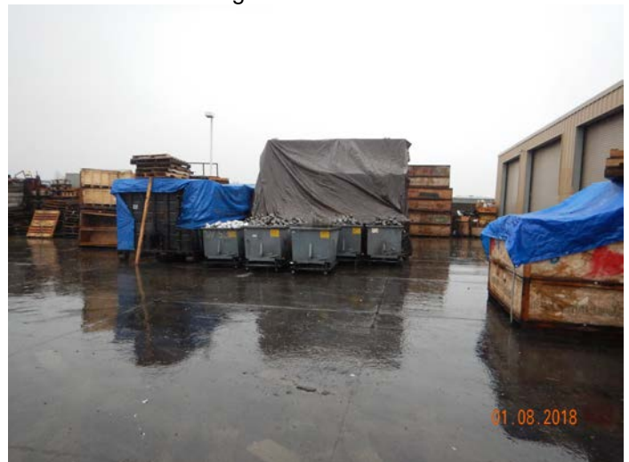
Photo 4. Uncovered bins of metal shavings and compressed shavings pucks during a rain event.
