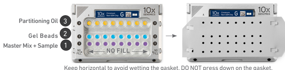
Keep horizontal to avoid wetting the gasket. DO NOT press down on the gasket.
