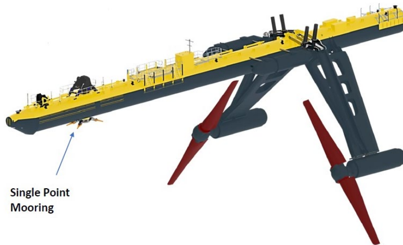
Figure 9. Single-Point Mooring Location on Orbital O2-X Hull
