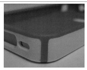
The side surfaces of the Rocon cases form a corner joint filled with the co-molded flexible inner layer which contributes to the overall flexibility of the case and which creates a stretch-zone that allows the case to deform to accept insertion of the phone.
