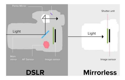
12. The absence of a mirror increases the camera's speed and allows it to be smaller and lighter than a traditional digital camera ("DSLR" or digital single-lens reflex camera).
