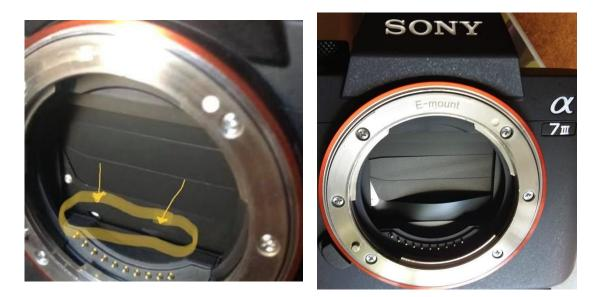
24. When a user removes the lens, the shutter is closed and stuck.
