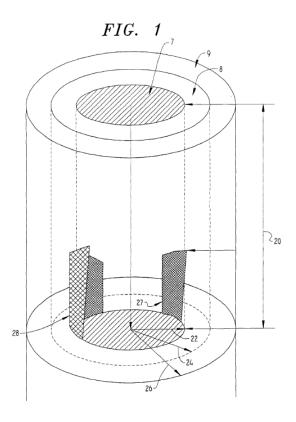
Figure 1, above, illustrates a longitudinal cross-sectional view of a coated optical glass fiber 7 coated with an inner primary coating 8 and a commercially available outer primary coating 9. *Id.* at 8:8-9; 10:7-9.
