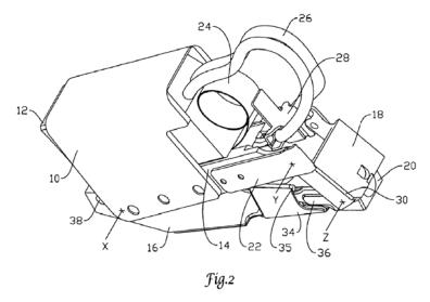
As illustrated in Figure 2 above, a hinging action takes place at certain pivot lines, such as pivot line "X," about which beam 14 moves with respect to lower
