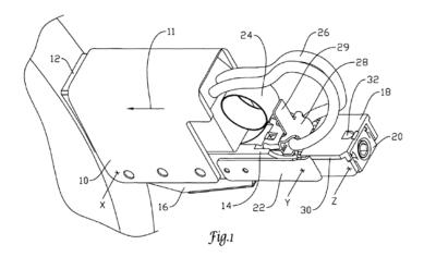
According to Figure 1 above, brush box 10 is affixed to beam 14, which is affixed, via a hinged attachment, to the lower mount block 16. *Id.* at col. 4, ll. 34–41. In the "engaged" position, a conductive path is formed from brush 12 through brush conductor 26, terminal 28, and conductor strap 34 (shown in Figure 2, reproduced *infra*). *Id.* at col. 7, ll. 10–14.
