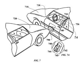
Figure 7, with Figure 7A inset, depicts vehicle 720 approaching the side of another vehicle 710 and shows transmitter 730 and receivers 734 and 736. Ex. 1001, col. 9, ll. 48-52; col. 18, ll. 28-40. Figure 7A provides a detailed view of the electronics that drive transmitter 730 and circuitry 744 containing neural computer 745 to process signals reflected or received from the external object using pattern recognition. *Id.* at col. 18, ll. 33-40.
