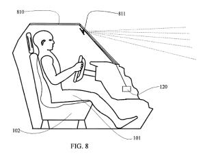
Figure 8 depicts a system for detecting the headlights or taillights of other vehicles used in conjunction with an automatic headlight dimming system. Ex. 1001, col. 9, ll. 54-58. CCD array in Figure 8 is designed to be sensitive
