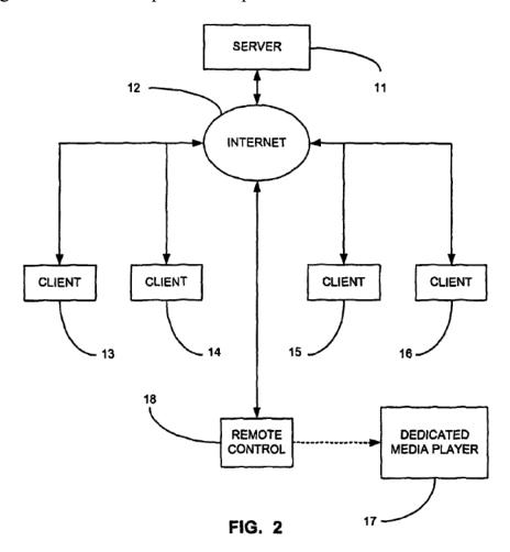
Figure 2 depicts an embodiment of the invention with a playlist communicated from server 11 to remote control 18 via Internet 12. Ex. 1001, 9:1–23. After the
