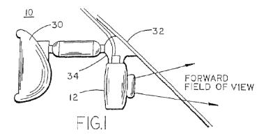
Figure 1 shows headlight dimming control 12, rearview mirror 30, windshield 32, and bracket 34. *Id.* at col. 3, ll. 58–60; col. 4, ll. 19–23. The '664 patent discloses that bracket 34 may fixedly mount imaging sensor module 14 "to, or near, the vehicle's windshield 32." *Id.* at col. 4, ll. 19–22.
