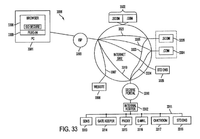
Figure 33 depicts an embodiment in which computer 3301 connects to secure server 3320 over Internet 3302, via the network that includes secure portal 3310.
