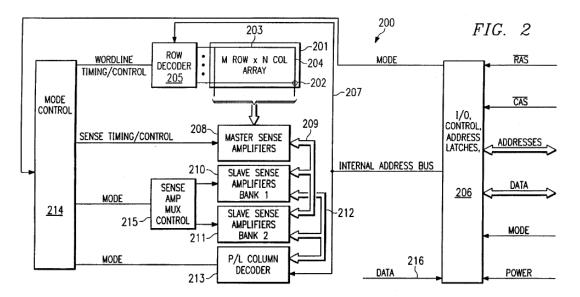
Figure 2 depicts a block diagram of memory system 200 with an M x N array of flash memory cells 201, with wordlines (rows) 203 and bitlines (columns) 204. *Id.* at 5:52–57, 3:25–26. Representative memory cell 202 is located at the
