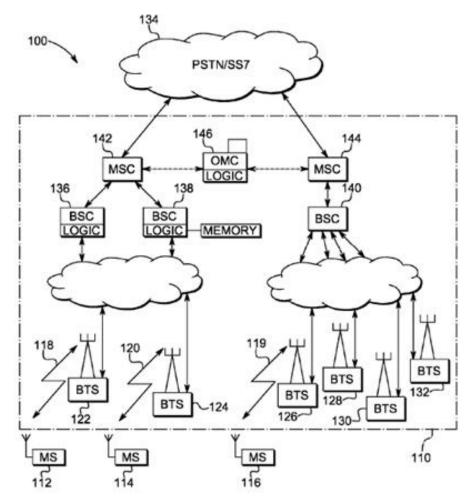
As shown in Figure 1, a plurality of subscriber terminals (*e.g.*, cell phones) 112, 114, 116 communicate wirelessly over radio links 118, 119, 120 with a plurality of base transceiver stations 122, 124, 126, 128, 130, 132, also known as "Node-Bs." Ex. 1001, 3:34–38. The cell phones and Node-Bs transmit and receive multi-rate signals. *Id.* at 4:39–44.
