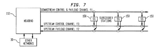
Figure 7 illustrates the three types of communication channels allocated by the network of the invention.
