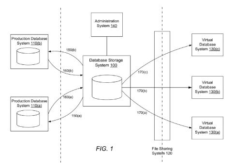
Figure 1 illustrates how information may be copied from production database systems 110 to database storage system 100. *Id.* at 7:12–15. To create a
