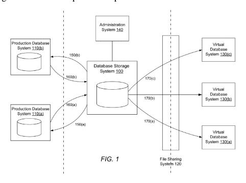
Figure 1 illustrates how information may be copied from production database systems 110 to database storage system 100. *Id.* at 7:12–15. To create a
