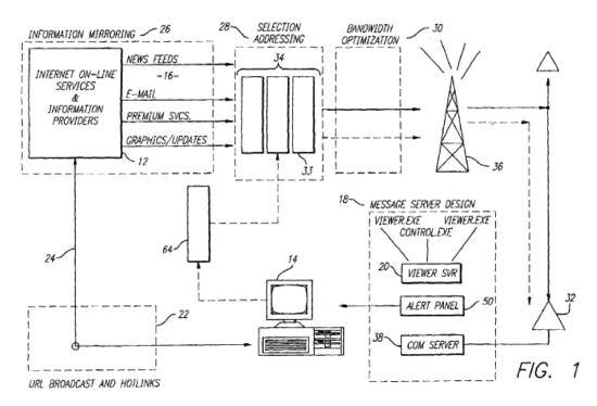
Figure 1 is a schematic diagram of a communication network. Once data is received at the user end, communications server 38 in message server design 18 notifies user interface panel 50, which presents an icon that, when clicked, notifies viewers 20 that are registered to display particular data on user computer 14 and alerts users to incoming messages. *Id.* at 6:52–62.
