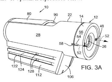
As shown in Figure 3A, digital video camera 10 comprises camera housing 22, rotatable lens 26, image sensor 18 (not shown), such as a
