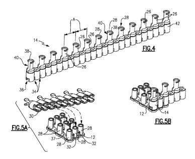
Figure 4 is a perspective view of an example pin bar. *Id.* at 1:65. Figure 5A is a perspective view of interfacing surfaces of an example base and the example pin bar. *Id.* at 1:66–67. Figure 5B is a perspective view of a pin bar mounted to an example base. *Id.* at 2:1–2.
