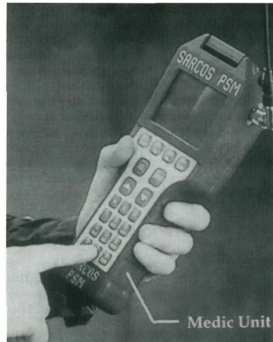
FIG. 1. The medic unit from the Sarcos, Inc. Personnel Status Monitor (PSM) system being developed for the military. (Courtesy of Dr. Stephen Jacobsen, Ph.D., Sarcos, Inc., Salt Lake City, Utah.)
