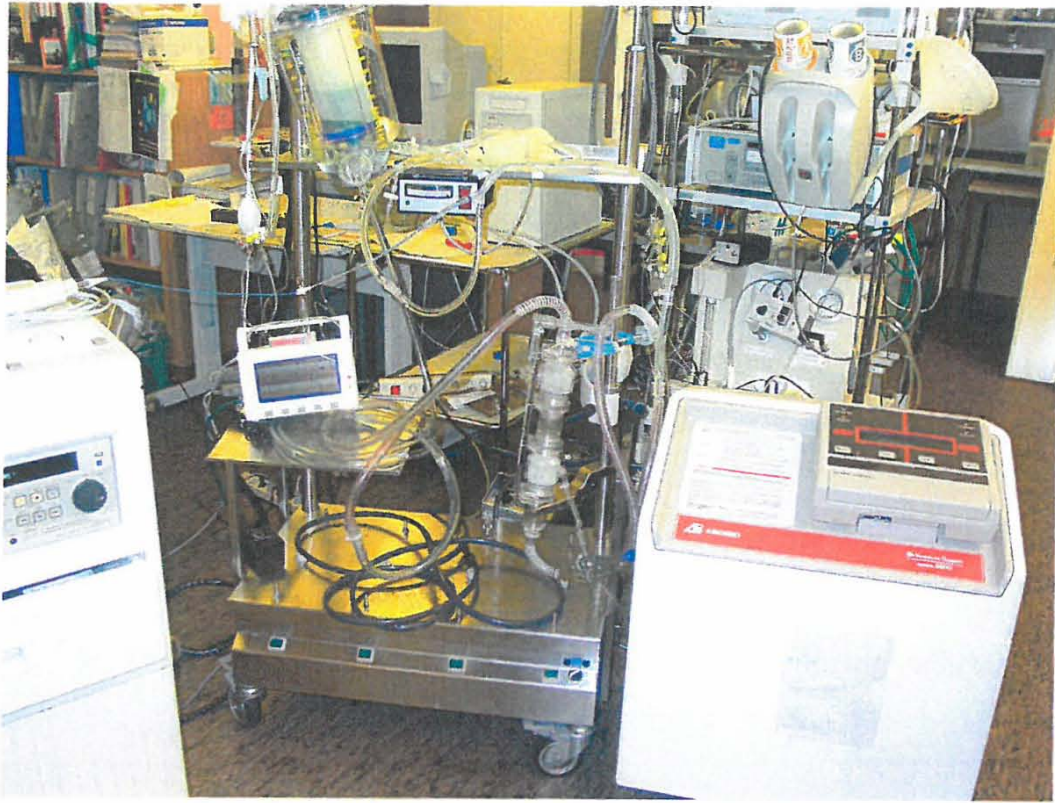
Fig 9. Mock loop device and the dynamic test of the valve
