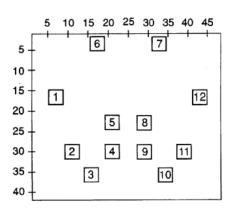
pressure sensors, arranged on the seat according to Figure 2, which is reproduced at left. *Id.* at 3:21-23. In this example, the sensors are turned on one at a time, a microprocessor samples each
