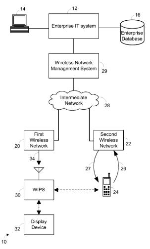
Figure 1 depicts wireless communication system 10 having enterprise information technology (IT) system 12 connected to one or more personal computers 14 and centralized enterprise database 16. *Id.* at 3:62–4:6. Enterprise IT system 12 uses wireless network management system 29 to communicate with first wireless network 20 and second wireless network 22 via intermediate network 28, which may be a wide-area network (WAN) or a local-area network (LAN). *Id.* at 4:34–41.
