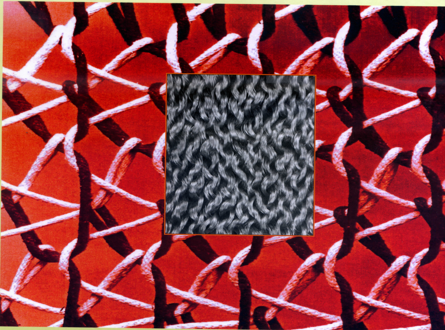
Crepe Americana Stitch Rope Model with photomicrograph of the fabric
