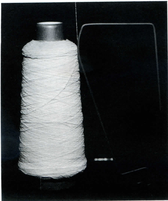
Fig. 25—The “Yarn Monitor” made by Stop-Motion Devices Corporation—another type unit that can be used successfully for tensioning yarn spun with a core of Blue “C” spandex on the side of the cone.
