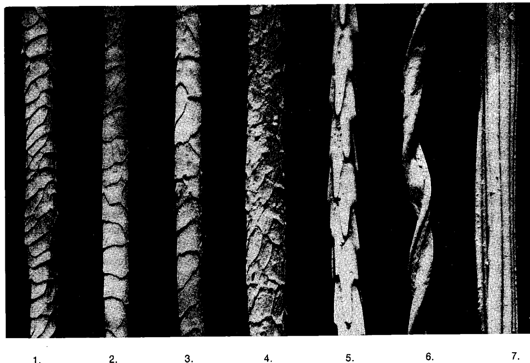
FIGURE 17.15 Surface of various fibers: 1. wool, 2. cashmere, 3. mohair, 4. camel, 5. mink, 6. cotton, 7. rayon (courtesy of Albany International).
