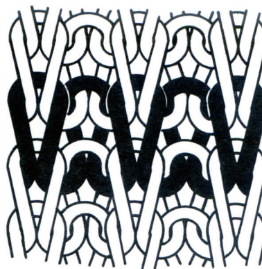
D. Spandex knitted in on a 1 x 1 rib fabric at predetermined course intervals.
