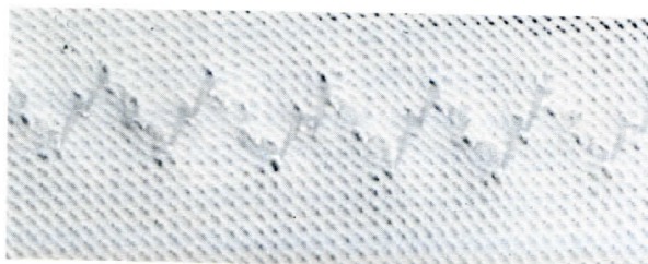
Fig. 87—A step zigzag (3 and 3) stitch should be used when more than 35 per cent stretch is required.
