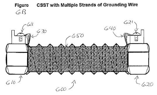
As shown in Figure 6B above, "CSST flex line 600 is shrouded by . . . wire mesh 650, which is attached to . . . collars 630, 640 on each end." *Id.* at 5:24–26. Also shown are "brass nuts 610, 620," which "have collars 630, 640 that protrude from the top." *Id.* at 5:22–24.
