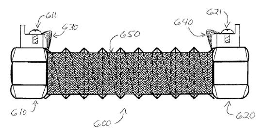
As shown in Figure 6B above, "CSST flex line 600 is shrouded by . . . wire mesh 650, which is attached to . . . collars 630, 640 on each end." *Id.* at 5:24–26. Also shown are "brass nuts 610, 620," which "have collars 630, 640 that protrude from the top." *Id.* at 5:22–24.
