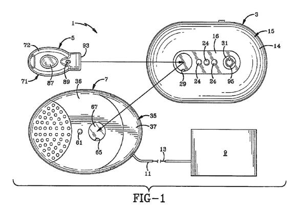
Figure 1 depicts security system 1 that includes programming station 3, programmable key 5, and alarm module 7 adapted to be attached to item of merchandise 9 by cable 11 with sense loop 13. *Id.* at 6:4–10. Programming station 3 randomly generates a unique security code (Security Disarm Code, or "SDC") that is transmitted via wireless (e.g., infrared) link to
