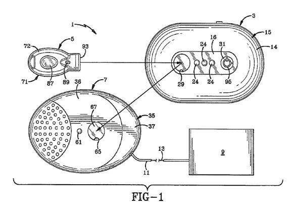
Figure 1 depicts security system 1 that includes programming station 3, programmable key 5, and alarm module 7 adapted to be attached to item of merchandise 9 by cable 11 with sense loop 13. *Id.* at 6:4–10. Programming station 3 randomly generates a unique security code (Security Disarm Code, or "SDC") that is transmitted via wireless (e.g., infrared) link to
