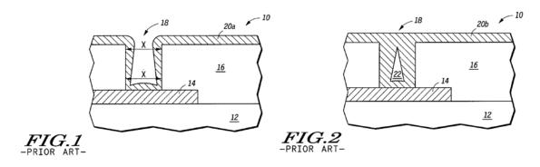
Figures 1 and 2 show, in cross-sectional diagrams, a method for forming a contact structure. *Id.* at 2:16–18. The top surfaces of dielectric layer 16 accumulate tungsten material 20a at a much faster rate than the bottom corners of contact opening 18. *Id.* at 1:46–48, Fig. 1. Due to this nonconformal deposition, the contacts end up with keyholes or voids 22. *Id.* at 1:59–61, Fig. 2.
