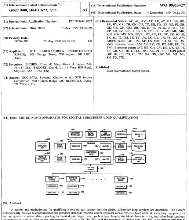
characteristics such as wire gauge, the presence of load coils (88, 90), and the presence of bridge taps (84, 86). The system determines which digital subscriber loop services are available for the copper loop based on the combination of all data obtained. The system may be implemented in part as an expert system with a knowledge base of qualification rules used in the decision-making process.
