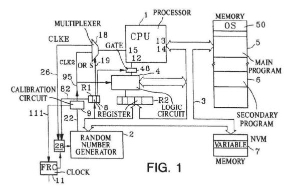
Figure 1 is a schematic diagram of electronic circuits of a microcomputer. *Id.* at col. 3, ll. 24–25.
