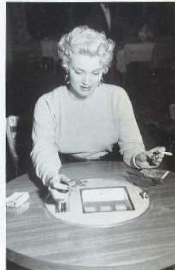
Introduced in 1954 at the Las Vegas Sands Hotel, the ROTO-SLOT, a circular cocktail table with a built-in Mills mechanism, could be played in six positions by lifting the knob on the right and rotating the playing unit. During the late 1950's and early 1960's built-in three reel slot bars were operating in Reno at the Golden Hotel and Mac's Club.
