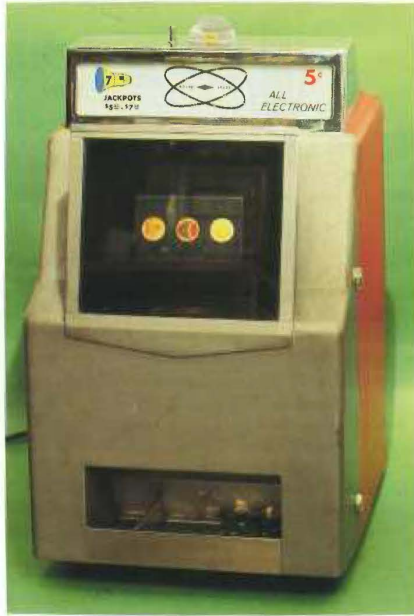
Rear projection read-out units were substituted for the mechanical reels on this first video slot. Only one handleless solid state prototype was constructed, unfortunately ahead of its time.
