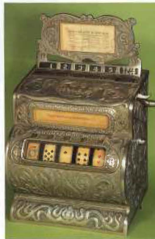
Caille 1905 HY-LOW The first coin played in the slot on the right spins all five reels, but on a second draw to revolve any other reel or reels to fill any particular hand, an extra coin has to be played in each slot which are numbered to correspond with each reel. Although, made for nickel play, they were also an ideal penny machine, as players will draw to more hands and take extra "chances."
