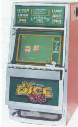
Built by Dale Electronics in Las Vegas, this was a complete dice game allowing up to 15 different bets to be made. The too-liberal solid state machine was abandoned due to poor "box hold," or net earnings.
