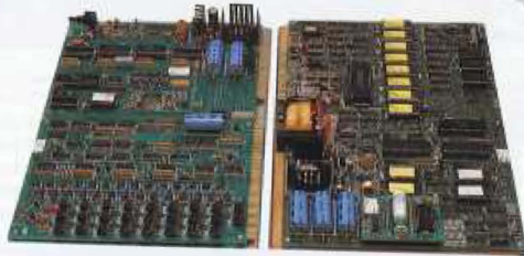
The microprocessor boards, right, control the operations of each poker hand.
