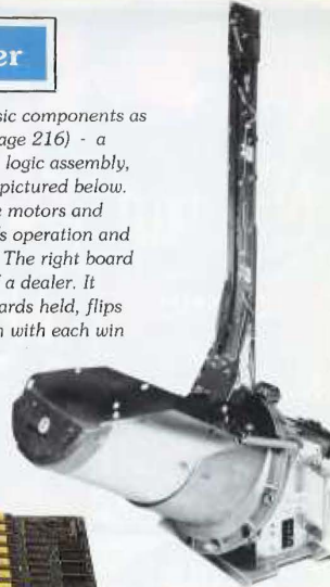
The hopper unit, above, controls the vital banking functions.
