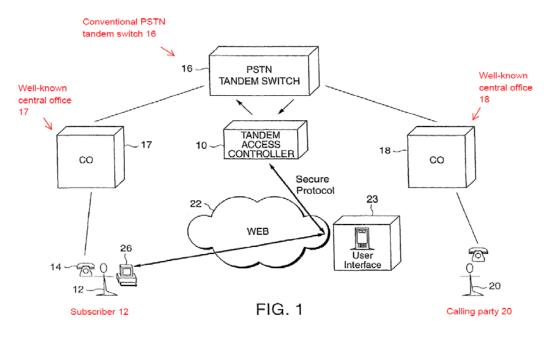
Annotated Figure 1 illustrates tandem access controller 10 connected to conventional PSTN tandem switch 16. *Id.* at 4:60–64. According to the '298 patent, "[d]etails of the operation of the existing phone network," including directing of phone calls by "existing" PSTN tandem switch 16 to central offices 17, 18 are further described in a publication incorporated by
