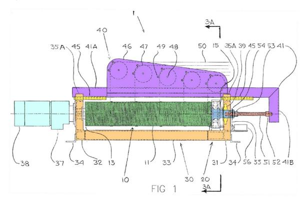
The colorized version of Figure 1 is a side view of an exemplary embodiment of the claimed winch system with some internal structures shown in dashed lines.
