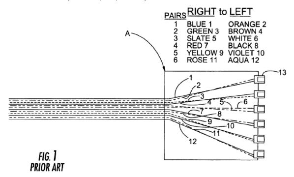
The patents explain that Figure 1 "illustrates a conventional module 'A' having six fiber pairs matched as follows: 1–2; 3–4; 5–6; 7–8; 9–10; and 11–12." *Id.* at 1:47–49. The patents explain that "[m]odule A is used in a system utilizing an 'A' and 'B' type module approach where the fibers in the 'B' module are flipped with respect to module A to address, or correct for, fiber polarity." *Id.* at 1:53–56.
