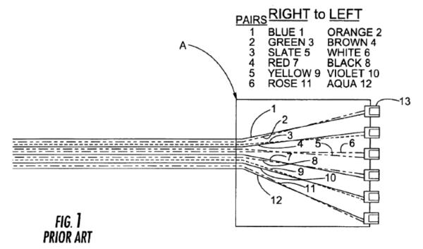
The patents explain that Figure 1 "illustrates a conventional module 'A' having six fiber pairs matched as follows: 1–2; 3–4; 5–6; 7–8; 9–10; and 11–12." *Id.* at 1:47–49. The patents explain that "[m]odule A is used in a system utilizing an 'A' and 'B' type module approach where the fibers in the 'B' module are flipped with respect to module A to address, or correct for, fiber polarity." *Id.* at 1:53–56.
