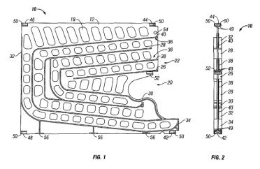
Figure 1 of the '111 patent "is a side view of a panel" (*id.* at 1:66–67), and Figure 2 is "an edge on view of a panel" (*id.* at 2:1–2). As shown, panel 10 is the "main element of the multi-chute gravity feed dispenser display" and
