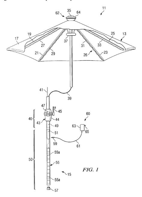
Figure 1 depicts the lighted umbrella with motorized opening and closing system according to the invention. *Id.* at 2:29–31. Umbrella apparatus 11
