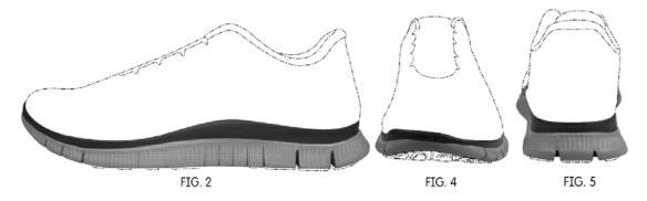
Figure 2 is a lateral side view of a shoe sole, and Figures 4 and 5, respectively, are front and rear views thereof. *Id.*
