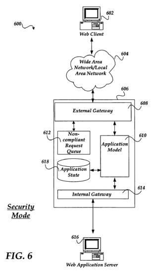
*Id.* at Fig. 6. Figure 6 is a functional block diagram of an embodiment of the invention operating in security mode. *Id.* at 8:63–64. As shown above in Figure 6, web application security system 606 is configured to intercept incoming messages from network 604 originating from web client 602, as well as outgoing messages from web application server 616. *Id.* at 8:64–9:3.
