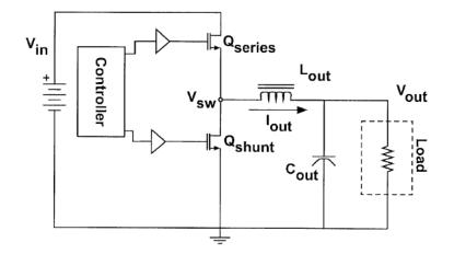
Figure 2 depicts a conventional switched mode regulator having transistor  $Q_{series}$  and transistor  $Q_{shunt}$  connected at common switching node  $V_{sw}$ .
