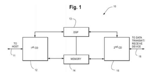
As shown in Figure 1 above, interface device 10 connects to a host device via host line 11, and to a data transmit/receive device via output line
