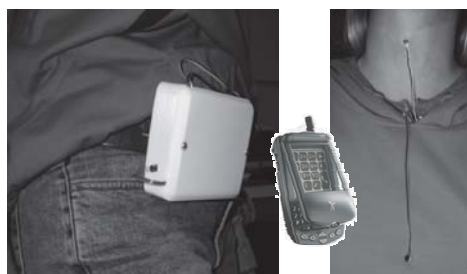
Figure 1. SenSay: sensor box mounted on the hip (left), the mobile phone (center), and voice and ambient microphones mounted on the user (right).
