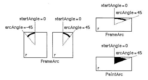
Figure 21. Operations on Arcs and Wedges
