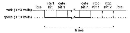
Figure 1. Asynchronous Data Transmission
