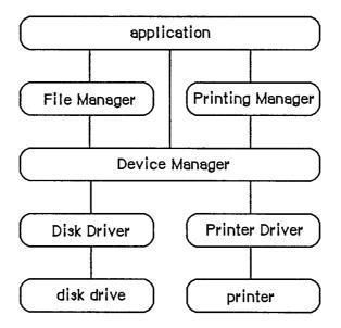
Figure 1. Communication with Devices
