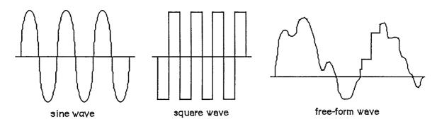
Figure 2. Types of Waveforms
