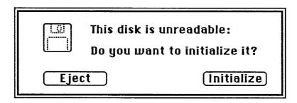
Figure 1. Disk Initialization Dialog for IOErr
