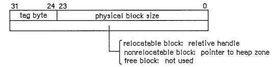
Figure 12. Block Header
