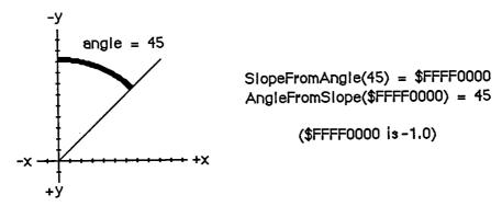
Figure 5. SlopeFromAngle and AngleFromSlope
