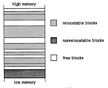
Figure 1. Fragmented Heap
