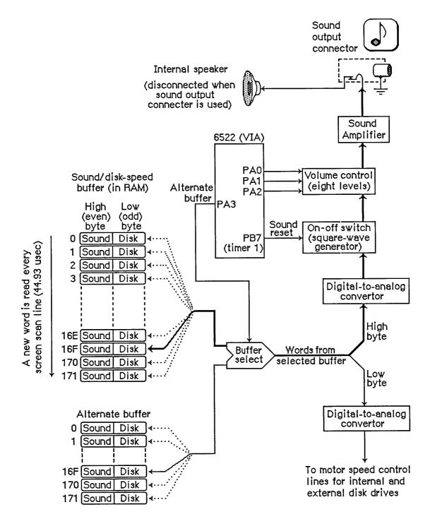
Figure 2. Diagram of Sound Port
