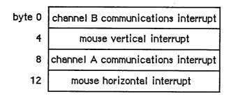
Figure 7. Level-2 External/Status Interrupt Vector Table
