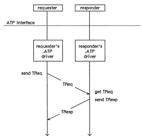
Figure 2. Transaction Process
