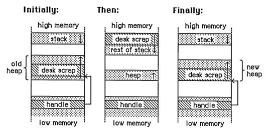
Figure 1. The Desk Scrap at Application Startup
