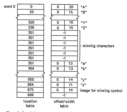
Figure 9. Sample Location Table and Offset/Width Table
