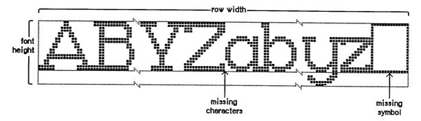
Figure 8. Partial Bit Image for a Font
