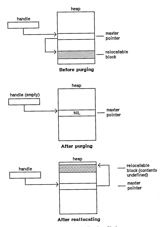
Figure 7. Purging and Reallocating a Block
