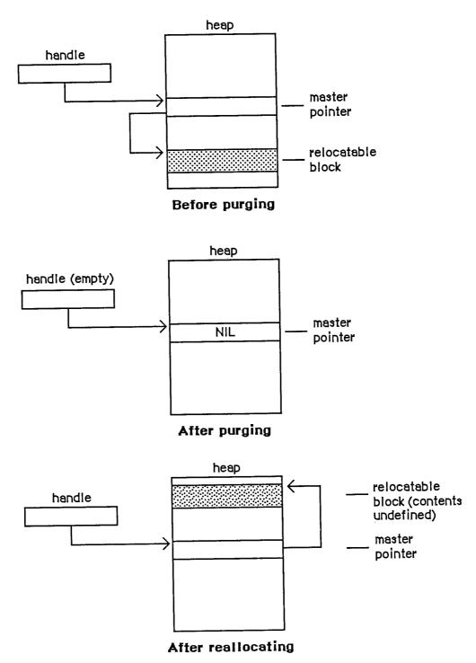
Figure 6. Purging and Reallocating a Block
