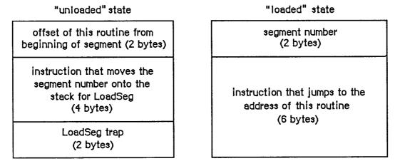
Figure 2. Format of a Jump Table Entry
