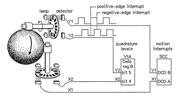
Figure 5. Mouse Mechanism
