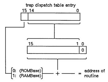
Figure 1. Trap Dispatch Table Entry
