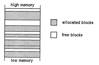
Figure 2. A Fragmented Heap
