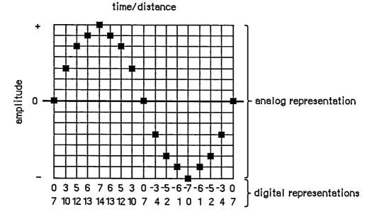
Figure 3. Analog and Digital Representations of a Waveform
