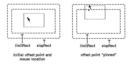
Figure 11. DragGrayRgn Operation on a Rectangular Region
