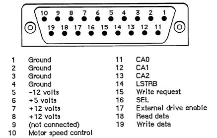
Figure 10. Pinout for Disk Jack
