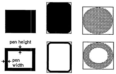
Figure 16. Solid Shapes and Framed Shapes
