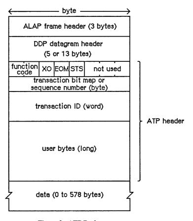
Figure 9. ATP Packet
