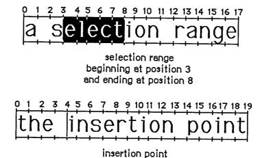
Figure 2. Selection Range and Insertion Point
