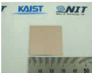
Fig. 1 inch size monolayer graphene substrate
