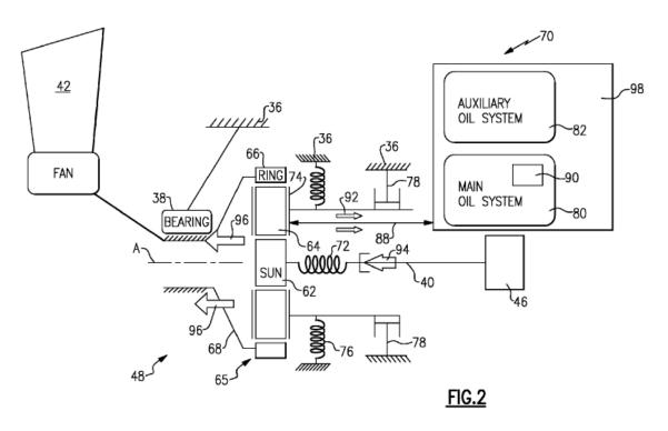
Figure 2 of the '943 patent, above, depicts gear assembly 65 with input shaft 40 and sun gear 62 driving intermediate gears 64, which in turn intermesh with ring gear 66 to drive fan 42. *Id.* at 5:61–6:2. Lubrication system 98, through main oil system 80, supplies lubrication to gears 62, 64, and 66 and in doing so, also cools the gears by removing heat generated in gear assembly 65 via line 88.<sup>1</sup> *Id.* at 6:28–40.
