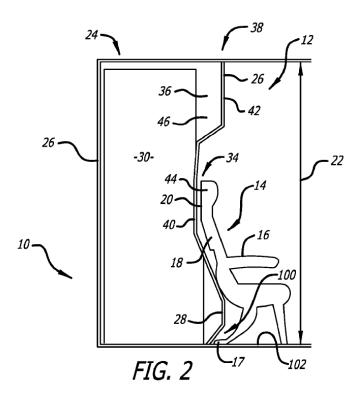
Figure 2, reproduced above, illustrates enclosure 10, such as a lavatory, positioned aft of aircraft cabin 12. Ex. 1001, 4:1–3, 4:8–13. The lavatory has walls that define interior lavatory space 30. *Id.* at 4:15–24. Forward wall 28 of the lavatory is described as "substantially not flat in a
